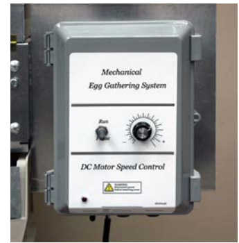
Egg flow to the table is controlled by a run/pause toggle switch and a belt speed adjustment knob.
