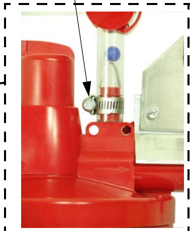
Figure 2.Lubricate O-Rings and attach Stand-Tube
