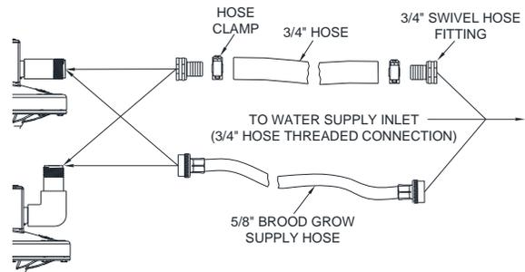
Figure 4. Water Supply Connection
