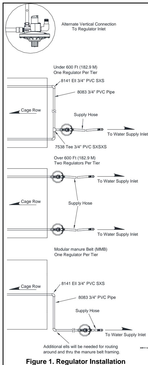
Figure 1. Regulator Installation
