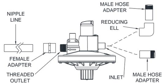
Figure 2. Water Line Connection
