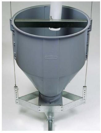
Two flattened areas (one on each side) are built in for panel type switch mounting.
