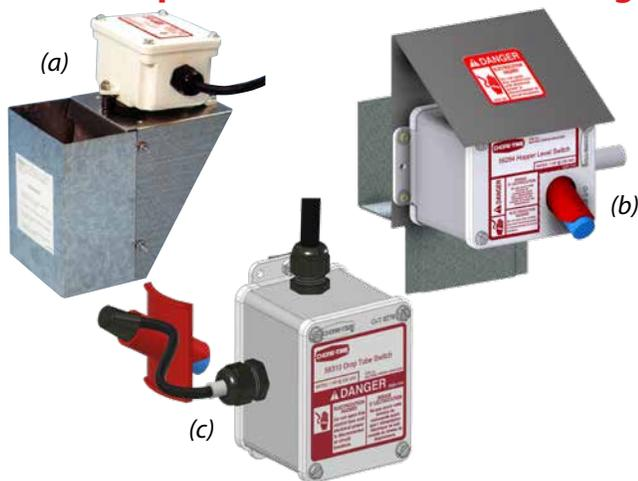
The mechanical Hopper Level Control (a) is used to maintain the feed level in the hoppers for continuous feed supply. The electronic Hopper Level Control (b) and Drop Tube Switch (c) adjust automatically to changes in feed type. A built-in programmable delay prevents short-cycling.
