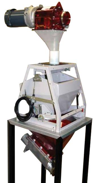
Chore-Time's Feed Scale is a diagnostic tool to help measure bird performance based on eating rates and habits.
