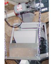
Chore-Time's Feed Scale helps with feed scheduling and measuring bird performance based on eating habits. Unique pivoting split hopper dumps feed from one side while the other side is filling for continuous flow.
