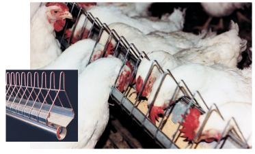
Chore-Time's ULTRAFLO® Breeder Feeding System quickly and reliably delivers uniform feed to every breeder hen. A variety of grill spacings and profiles is available to prevent males from eating the hens' ration
