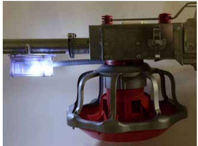
Chore-Time's Feeder Control Pan Light attracts birds to the control pan. Available for the REVOLUTION® Feeder (shown) and other Chore-Time® Feeders. Can also be retrofitted to a variety of feeding systems.
