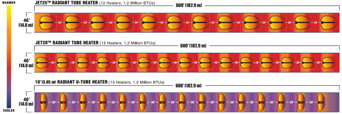
$JET^{M}$  Heaters provide even heat along the full length of the house. With traditional 40- and 50-foot (12.19- and 15.24-meter) tube heaters, floor temperatures decline rapidly along the tube length, producing arrowhead-shaped floor heat patterns.
