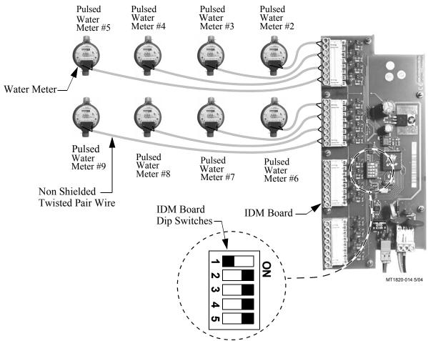
Using the blue and brown wires from the Feed Scales Connect Feed Scales #2 through #9 to the IDM board terminals using Twisted Pair Wire (See Figure below). Note the correct position of the Dip Switches. See Feed Scale Manual MT1811 for additional information if needed.
