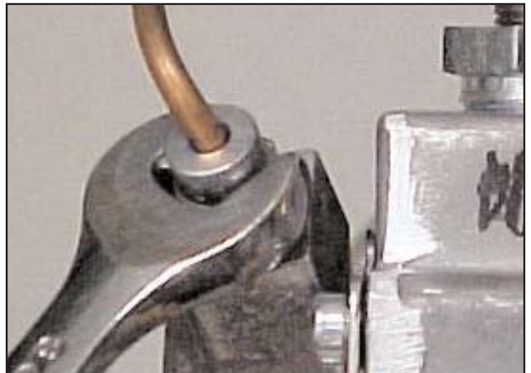
(13) Attach THERMOCOUPLE to CONTROL VALVE . Finger tight plus 1/4 turn to avoid damaging ceramic.
