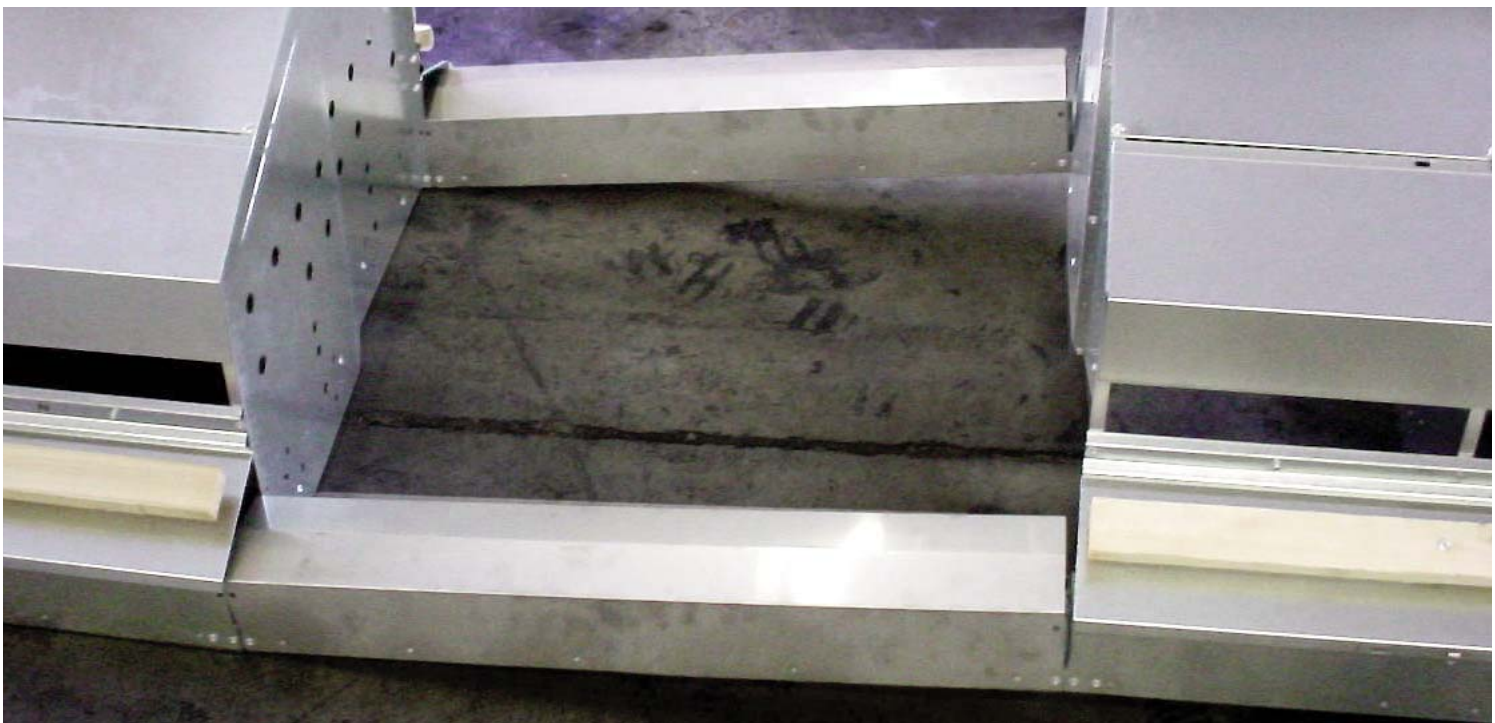
Illustration of a 2 Rivet connection per end of passageway to permit line flex.
