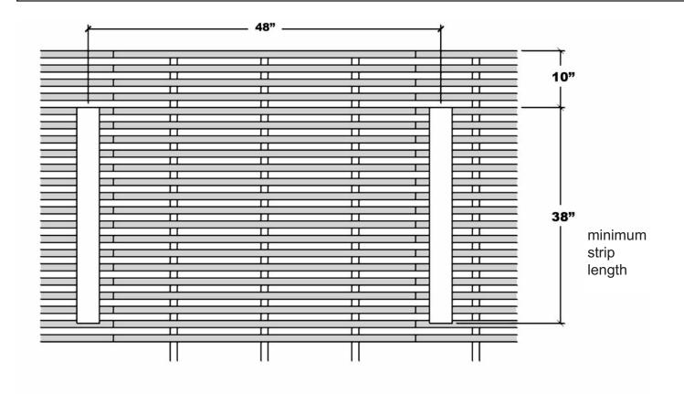
8' SECTION PLACEMENT OF 1 x 4 x 38 STRIPS
