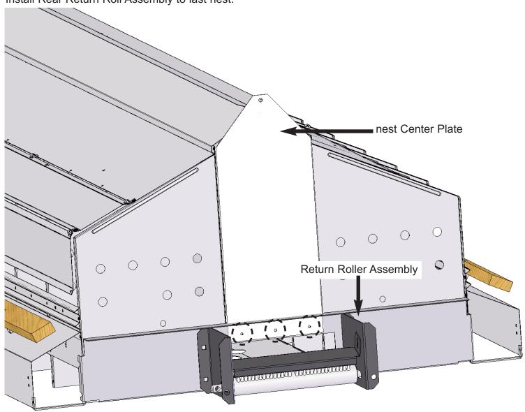
Attach the End Roller Assembly to the nest Center Plate using Pop Rivets via the three holes shown in the illustration above. Dust cover removed for clarity.
