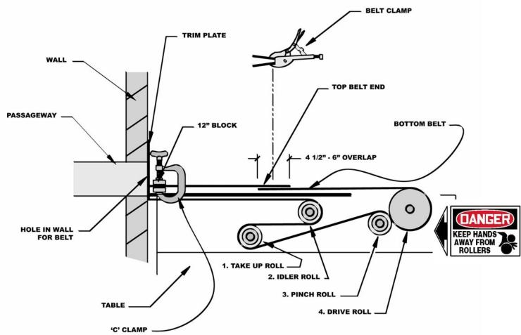
NOTE: DO NOT OVER TIGHTEN THE BELT. An over tightened belt causes decreased belt life, poor performance and excessive wear on the drive system. The belt may become cupped and allow eggs to go underneath it. The belt may become permanently creased. The belt should be pulled snug and slightly stretched, using the method described here.
