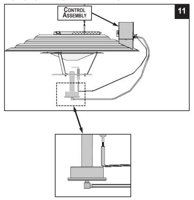
12. Suspend the brooder: to level the brooder simply support the heater underneath and then move the s-hook forward or backward. After it is level clamp both ends of the s-hook shut. The brooder should hang with the control assembly tilted slightly downward. Normally the brooder is attached to a winch cable used for raising and lowering.
