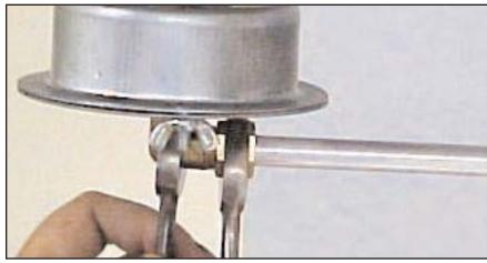
**STEP 12**: Insert one end of pilot tubing into orifice on burner pan. Insert other end in control assembly. Use two wrenches to tighten comp nut to avoid damaging tubing.
