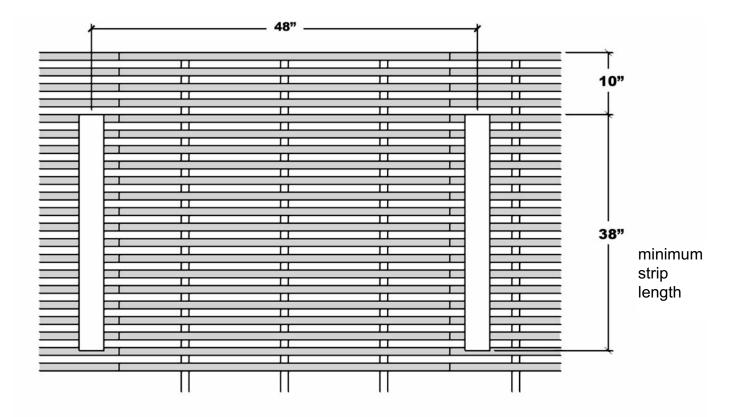
8' SECTION PLACEMENT OF 1 x 4 x 38 STRIPS
