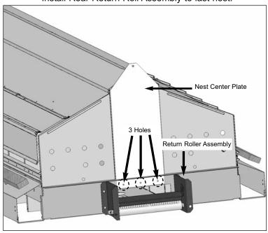
Attach the End Roller Assembly to the nest Center Plate using Pop Rivets via the three holes shown in the illustration left. Dust cover removed for clarity.
