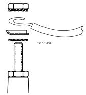
Conduit Entry should be at opening(s) provided or at location(s) indicated by dimples on outside of enclosure. Conduit hubs must be CSA certified and should be suitable for the application. If required to make field connections to stud type terminals, use hardware provided and assemble as shown.
