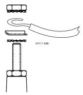
Conduit Entry should be at opening(s) provided or at location(s) indicated by dimples on outside of enclosure. Conduit hubs must be CSA certified and should be suitable for the application. If required to make field connections to stud type terminals, use hardware provided and assemble as shown.
