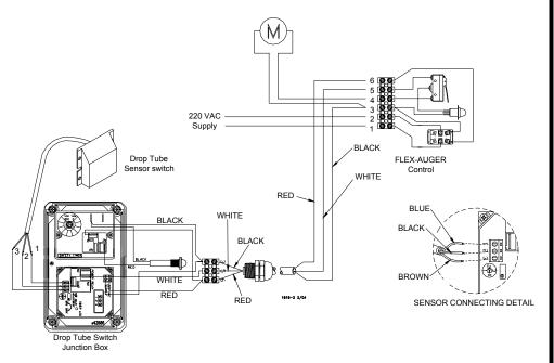
49264 Drop Tube Switch Wiring Diagram
