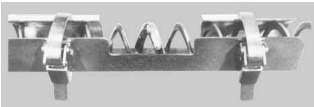
Figure 14. Clamping Auger in Place Using a Brazing Clamp
