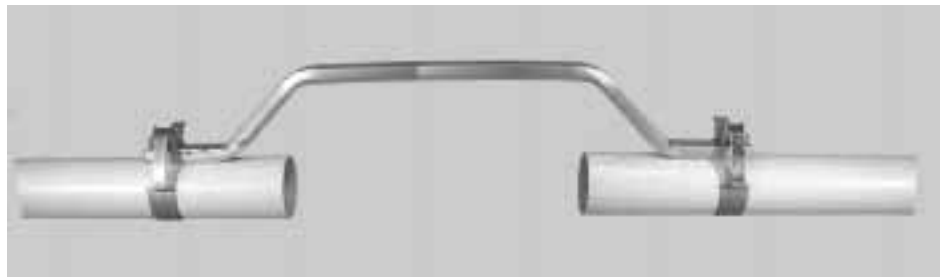
Figure 6. Welding Bridge attached to Tube
