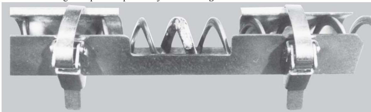
Figure 16. Clamping Auger in place using a Brazing Clamp.
