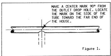
Center the 23877 Drop Mount Plate Assembly over the mark. Clamp the Drop Mount Plate on the tube so that the stud in the plate is horizontal. See Figures 2 and 3.
