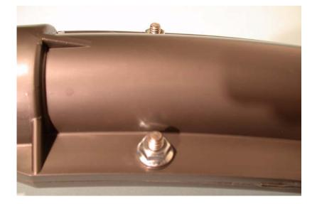
Slide the steel connecting tube in the adapter,. secure the tube using a adjustable clamp. see photo at the side. Note: The steel tube will be used to connect the two elbows.
