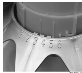
Figure 49. Feeder Pan Assembly adjustment
