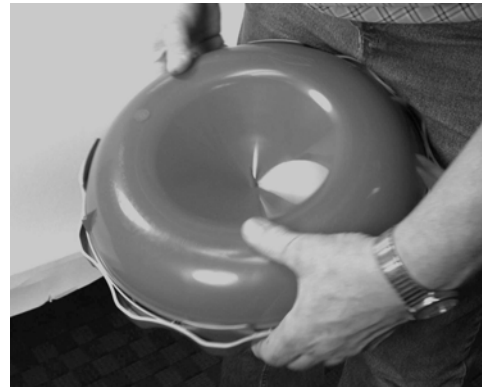
Figure 24. Assembling Support Cord to Feed Cone
