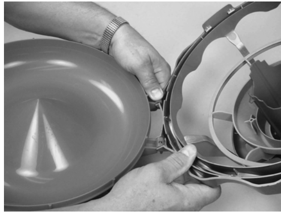
Figure 23. Assemble the grill ass'y to the feeder pan
