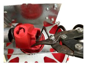
**Step 5.** Slid the new Cone/Grill/Pan assembly on to the Stub Tube (**Item 1**) as shown, and slide the new Top (**Item 2**) into place. ENSURE HOLE IN NEW CONE IS ON THE SAME SIDE AS THE WHITE RELAY BOX BEFORE MOVING ON!!!!
