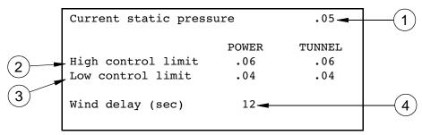
Figure 14. Static Pressure Screen
