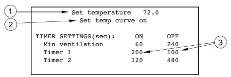
Figure 7. Model 16 Set Temp./Min. Timer Screen
