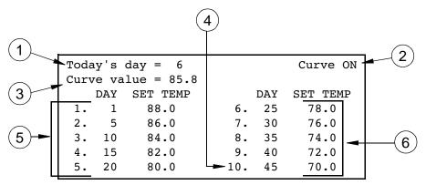
Figure 12. Set Temperature Curve Screen
