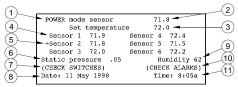
Figure 6. Model 16 Current Conditions Screen
