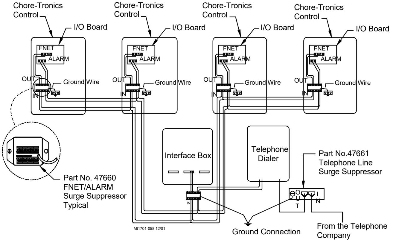
Note: There must be a ground rod within 10 ft. of the ground terminal of each surge suppressor. The wire size from the suppressor to the ground rod should be 12 gauge or larger.
