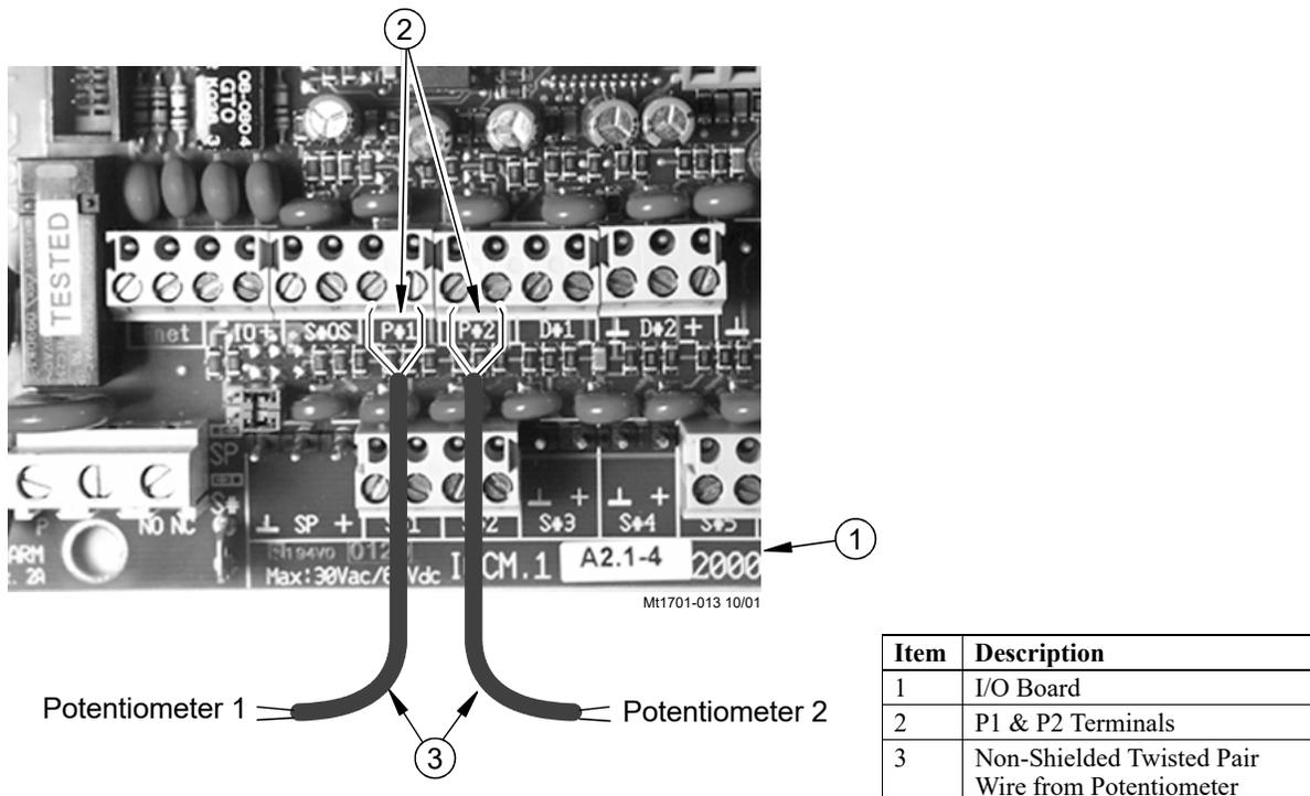
Figure 36. Potentiometer Wiring
