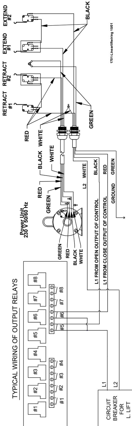
NOTE: THIS ASSUMES THE LINEAR LIFT OPENS THE INLET WHEN IT EXTENDS AND CLOSES THE INLET WHEN IT RETRACTS
