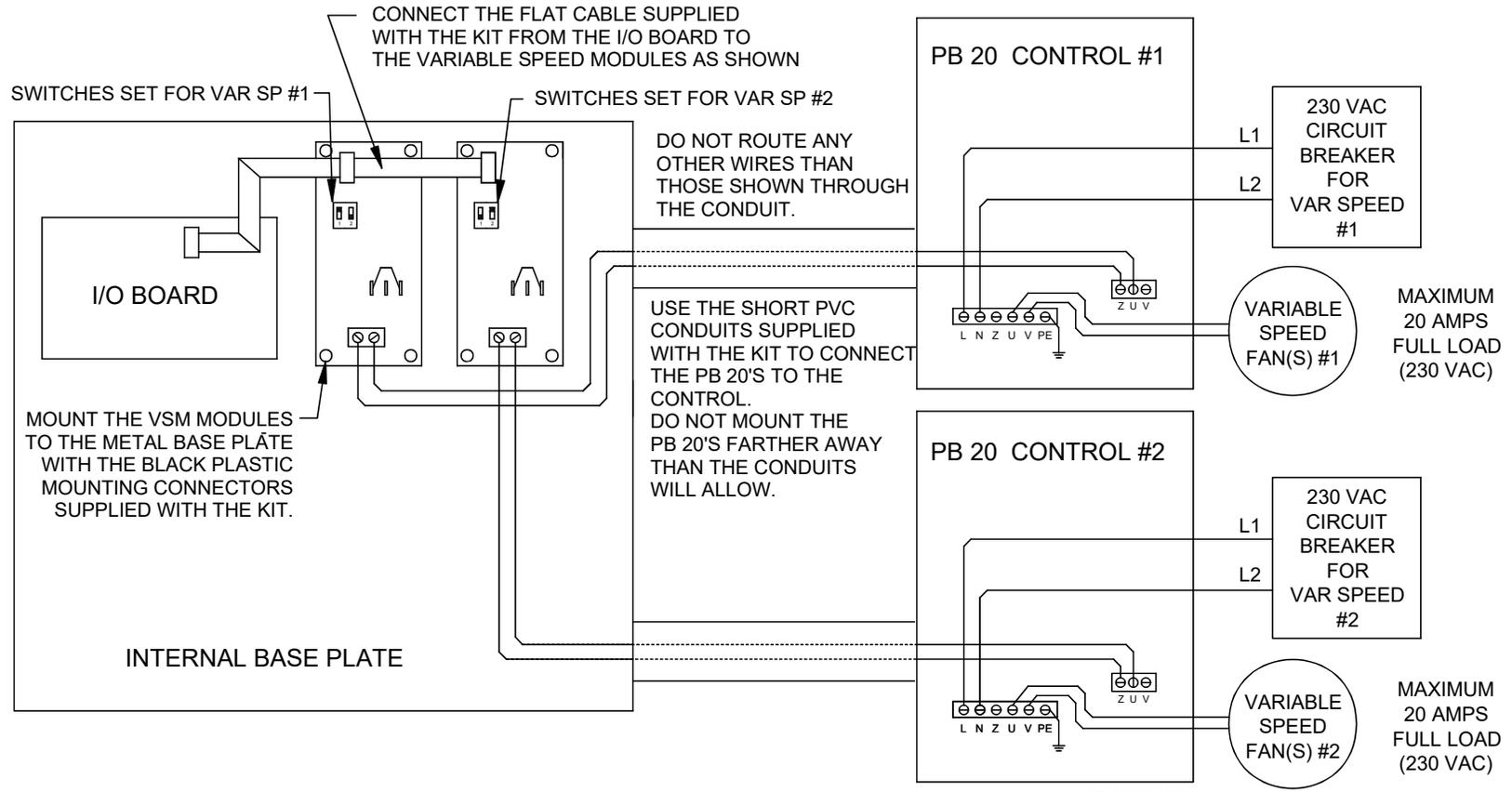
Figure 62. Variable Speed Kit 42522 Wiring
