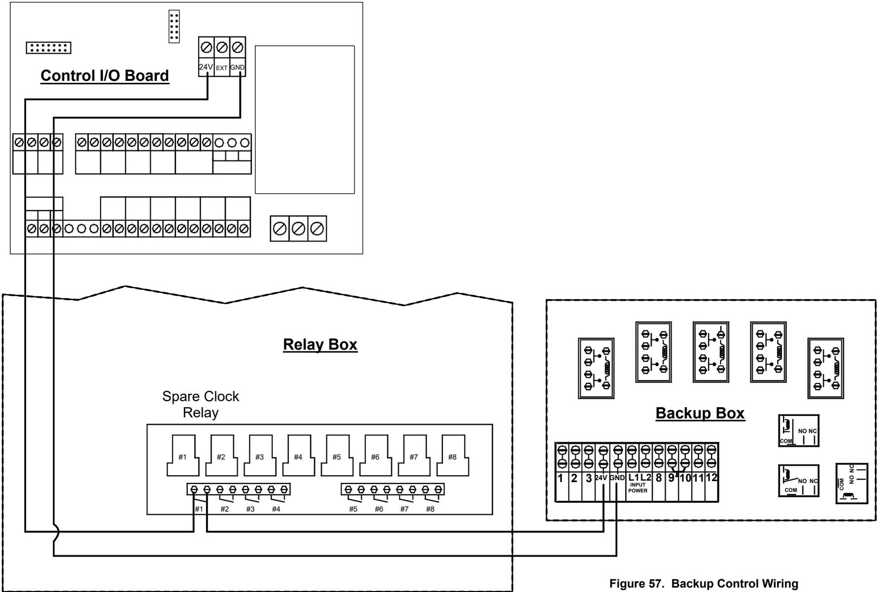
Figure 57. Backup Control Wiring
