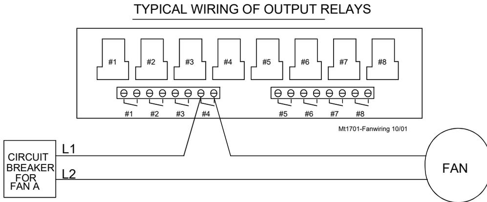
ALL OUTPUT RELAYS ARE SPST WITH DRY CONTACTS AS SHOWN. THIS SHOWS A TYPICAL SITUATION WHERE A FAN HAS BEEN ASSIGNED TO RELAY 4 IN THE SETUP SCREEN.
