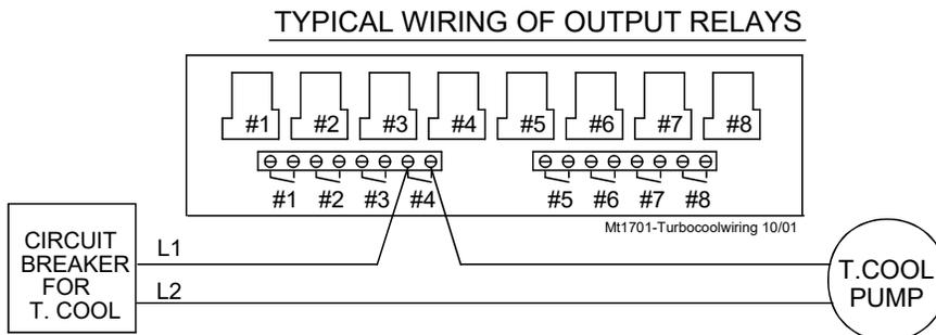
ALL OUTPUT RELAYS ARE SPST WITH DRY CONTACTS AS SHOWN. THIS SHOWS A TYPICAL SITUATION WHERE THE TURBO COOL PUMP HAS BEEN ASSIGNED TO RELAY 4 IN THE SETUP SCREEN.
