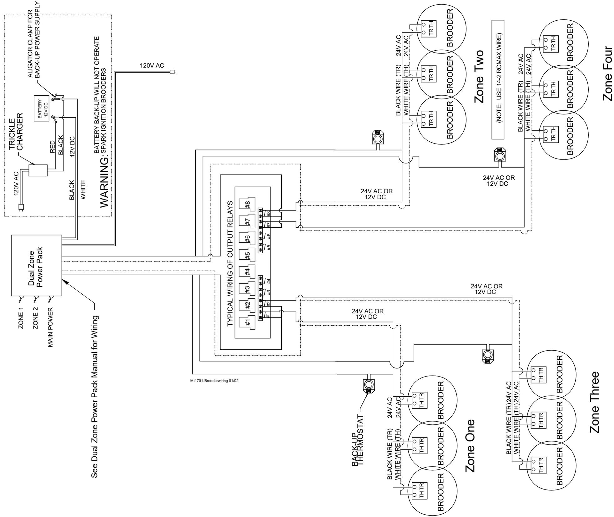
Figure 67. Brooder Wiring
