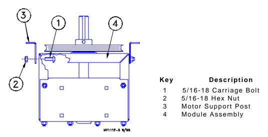
Figure 5. Fan Module installation (top view).
