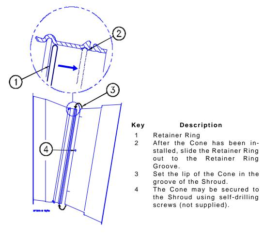
Figure 10. Cone Installation (side view).
