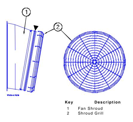
Figure 13. Shroud Grill installation
