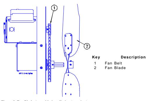
Figure 8. Fan Blade Assembly installation (top view).
