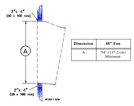
Figure 3. Wall opening requirements (side view).
