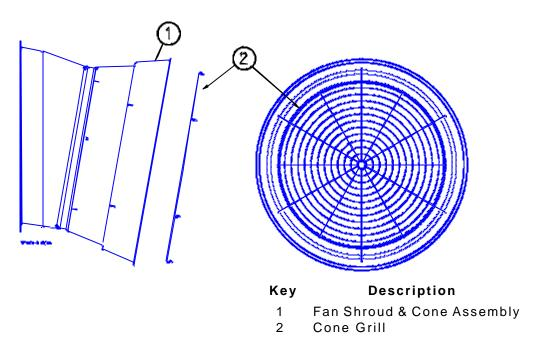
Figure 12. Cone Grill installation
