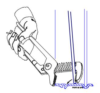
Figure 11. Seating the Retainer Ring in its final position (side view).
