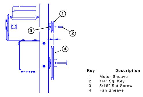
Figure 7. Motor Sheave installation (side view).
