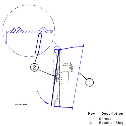
Figure 9. Retainer Ring Installation (side view).
