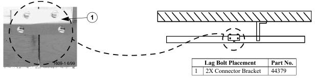
Figure 8. Connect 2 x 6's with 2X Connector Brackets
