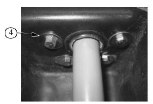
Figure 3. Inlet Pipe Support Installation
