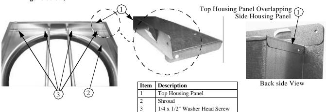
Now that all four Housing Panels are attached to the Shroud, Use four 1/4 x 1/2" Hex Washer Head Screws to attach all four Housing Panels together using the predrilled holes at the four Corners. (See Figure at right). Place the Fan Description Decal, (Item 4), (Included in the Parts Package) above the Danger Decal in the bottom corner of the Fan as shown.
