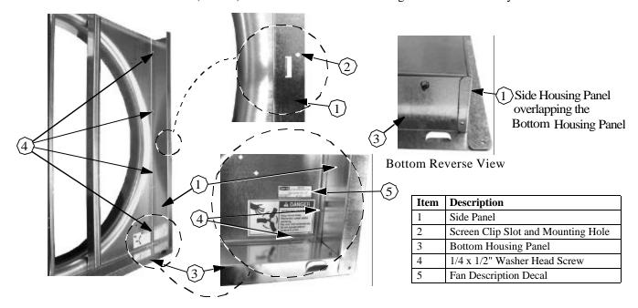
Attach the Top Housing Panel to the Shroud using the pre-drilled holes with four 1/4 x 1/2" Washer Head Screws. The Top Housing Panel should overlap the Side Housing Panels to provide water run-off. (See Figure below)
