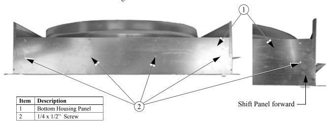
Remove the  $1/4 \times 1/2$ " Screws from the three remaining panels and shift them to the second set of holes and re-attach them to the shroud exactly the same as you did to the Bottom Panel. Attach the four Housing Panels together at the Corners of the Fan with four  $1/4 \times 1/2$ " Screws at the locations **shown below**. In total there should be 4 Screws holding each Panel to the Shroud and 4 Screws holding the Panels together at the Corners of the Fan for a total of 20.
