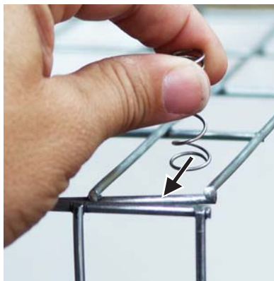
A) Slide a Spring (54480) over both Screen Panel Wires exactly as shown.
