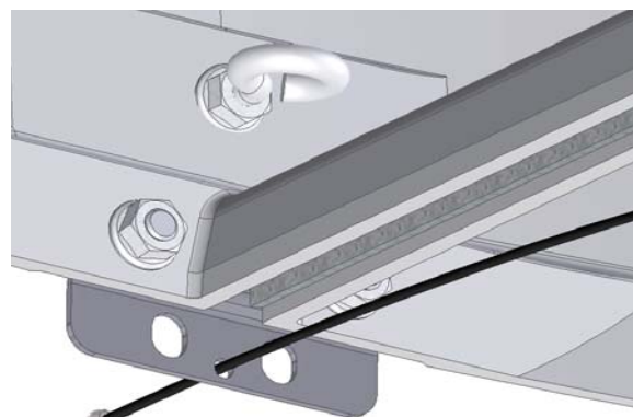
Insert (53399) Door Stop Cable Assembly into Top Pivot Plate
