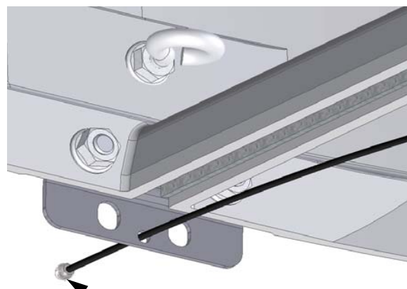
Insert (53399) Door Stop Cable Assembly into Top Pivot Plate
