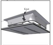
Attach string to Weight Arm with a regular knot. String should always be pulled parrallel with inlet when inlet is being pulled shut.
