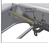
Hang S-hook into pre-drilled hole (A). Attach spring on S-Hook and J-Hook (B). Repeat for opposite side.
