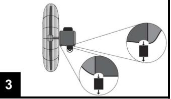
Attach fan to bracket. Insert bracket flag in between the motor flags and secure using the center holes on the motor flags with (1) 3/8" x 1-1/4" hex bolt, (2) 3/8" washers and (1) 3/8" nylock nut as shown in step 4a. Using the crescent openings on the motor flags, install the (1) 1/4" x 1" hex bolt, (2) 1/4" washers and (1) 1/4" nylock nut as shown in step 4b. Adjust the fan to the desired angle and tighten hardware to secure fan angle.
