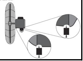
Attach fan to bracket. Insert bracket flag in between the motor flags and secure using the center holes on the motor flags with (1) 3/8" x 1-1/4" hex bolt, (2) 3/8" washers and (1) 3/8" nylock nut as shown in step 4a. Using the crescent openings on the motor flags, install the (1) 1/4" x 1" hex bolt, (2) 1/4" washers and (1) 1/4" nylock nut as shown in step 4b. Adjust the fan to the desired angle and tighten hardware to secure fan angle.
