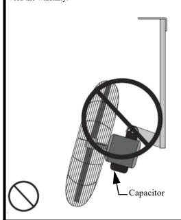
Do NOT mount bracket horizontally. The included bracket was not designed to be mounted this way and cannot withstand the structural stress caused by the weight and movement of the fan. Mounting the bracket and fan this way will void the warranty.
