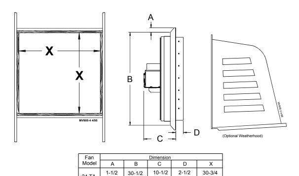
Figure 1. Fan and Framing Dimensions (side view)
