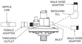
Figure 2. Water Line Connection
