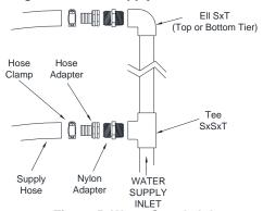
Figure 5. Water Supply Inlet
