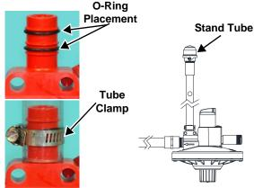
Figure 3. Stand Tube Installation
