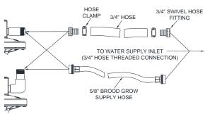
**Figure 4. Water Supply Connection**
