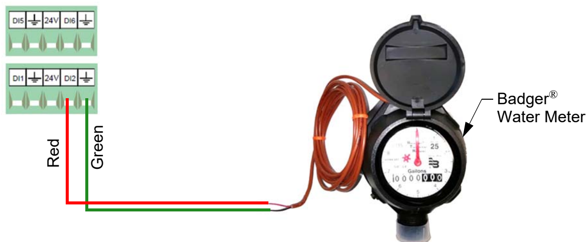
Figure 28. Water Meter Wiring
