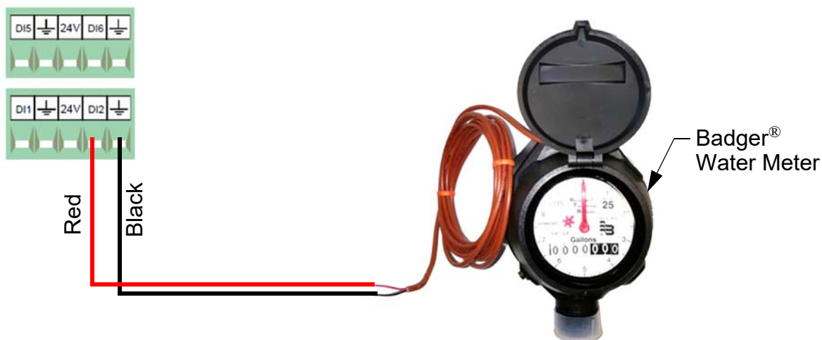
Figure 16. Water Meter Wiring
