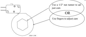
Figure 9. Linear Actuator Adjustment Procedure (side view)
