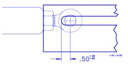
Figure 8. Linear Actuator Adjustment Procedure (side view)
