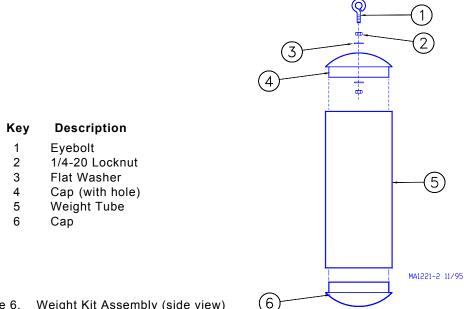
Figure 6. Weight Kit Assembly (side view)
