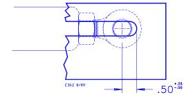
Figure 7. Linear Actuator Adjustment Procedure (side view)
