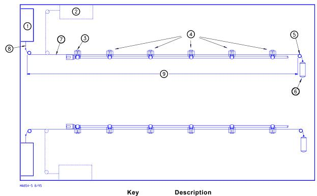
1 Linear Actuator 2 Linear Actuator (optional location) 3 **Drop Feeder Control Unit** 4 Drop Feeder 5 Pulley 6 Weight 7 1/8" (3.1 mm) Stainless Steel Cable 8 3/16" (4.7 mm) Stainless Steel Cable 9 200' (61 m) Maximum
