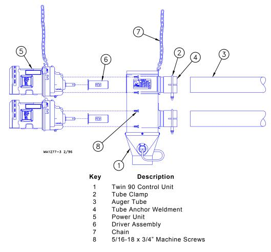
Figure 2. Power Unit and Auger Tube Installation (side view)
