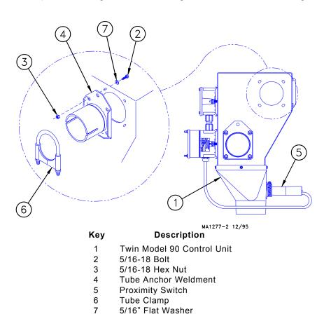
Figure 1. Tube Anchor Installation
