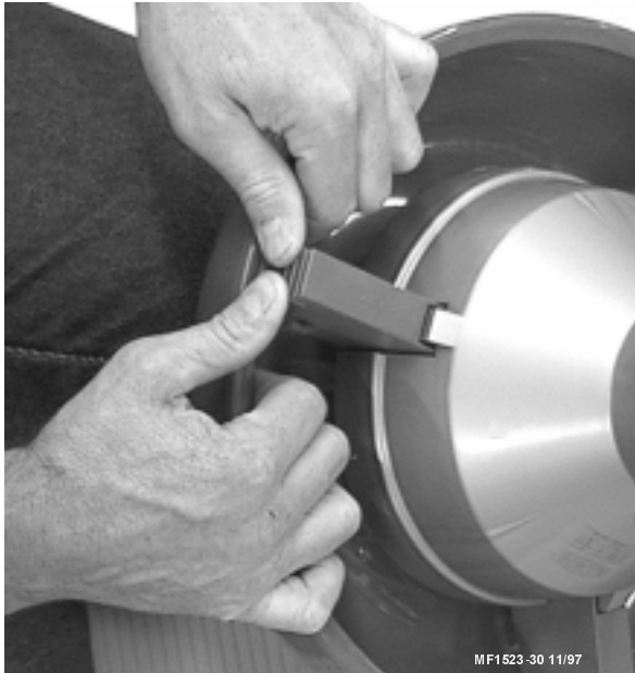
Figure 12. Assembling the center support and feed cone to the pan.
