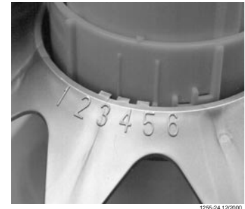
Figure 3. Feeder Pan Assembly adjustment
