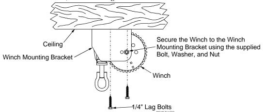
Figure 6. Winch Mounting
