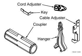
**Figure 9. Nipple Waterer Components**
