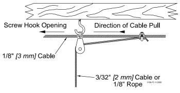
Figure 3. Screw Hook Installation
