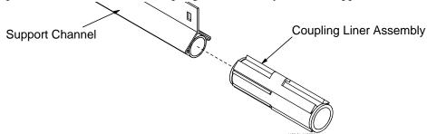
Figure 10. Coupling Liner Assembly Installation
