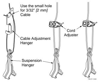
Figure 8. Cable Drop Installation
