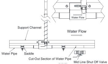
Figure 13. Mid Line Shut-Off Valve Installation
