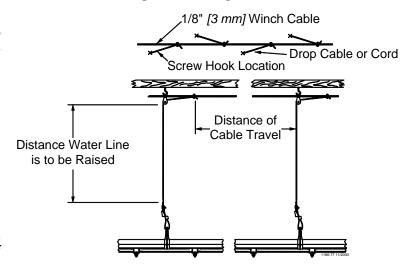
Figure 5. Offset the Screw/Ceiling Hooks
