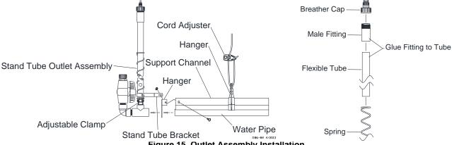
Figure 15. Outlet Assembly Installation
