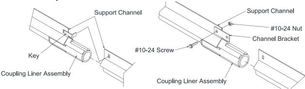
Figure 11. Securing the Water Line together
