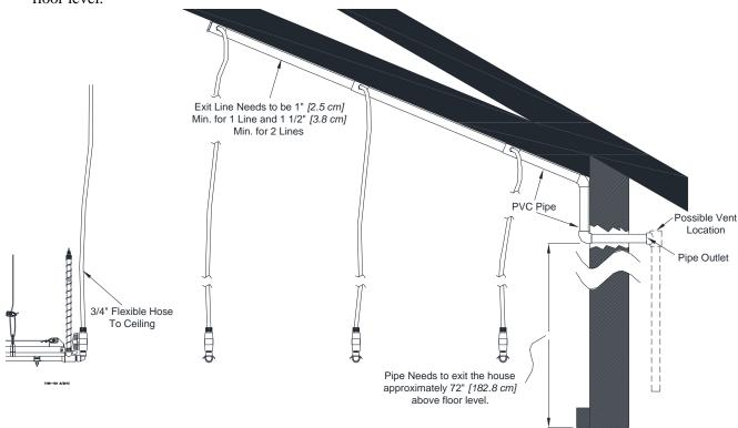
Figure 13. Flush System Component Layout Diagram
