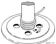
Figure 7. Cable Wrap on Drum
