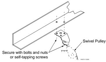
Figure 4. Ceiling Hook Installation
