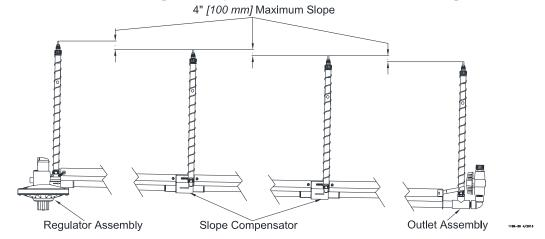
Figure 14. Slope Compensator Assembly Installation
