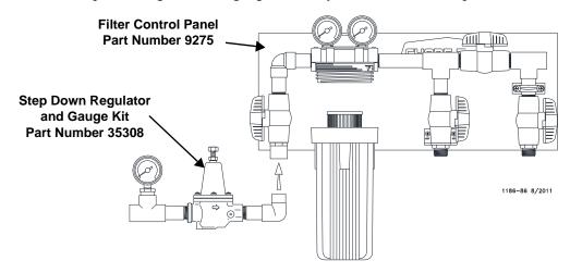
Figure 6. Control Panel Installation
