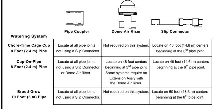
Begin at the Manifold end of the cage row. DO NOT INCLUDE THE CONNECTION AT THE MANIFOLD WHEN COUNTING PIPE JOINTS. Repeat the pattern specified above for the entire length of the cage row (on each tier).
