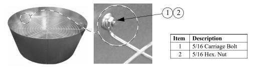
Use 5/16 Carriage Bolts and Flange Nuts to attach the Cone Brackets to the Fan Shroud as shown. Pick up the Cone and rest it on top of the Fan orifice. Line up the 5/16 Flange Bolt previously threaded into the Cone with the holes in the Cone Brackets and fasten with 5/16 Flange Nuts. Working around the Fan Orifice in a circular motion Slide the Cone over the Fan Orifice. The Cone will Fit snug. Use 5/16-18 Flange Nuts to secure the bottom of the Cone to the Cone Brackets.
