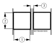
Planning the layout of the spacing between fans is very important. Spacing too close together will cause interference between Discharge Cones. Rough Openings for Fans are shown above.
