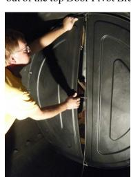
the Top Pivot Bracket lift it from the Bottom Pivot Plate and set aside somewhere safe to be reinstalled later.
