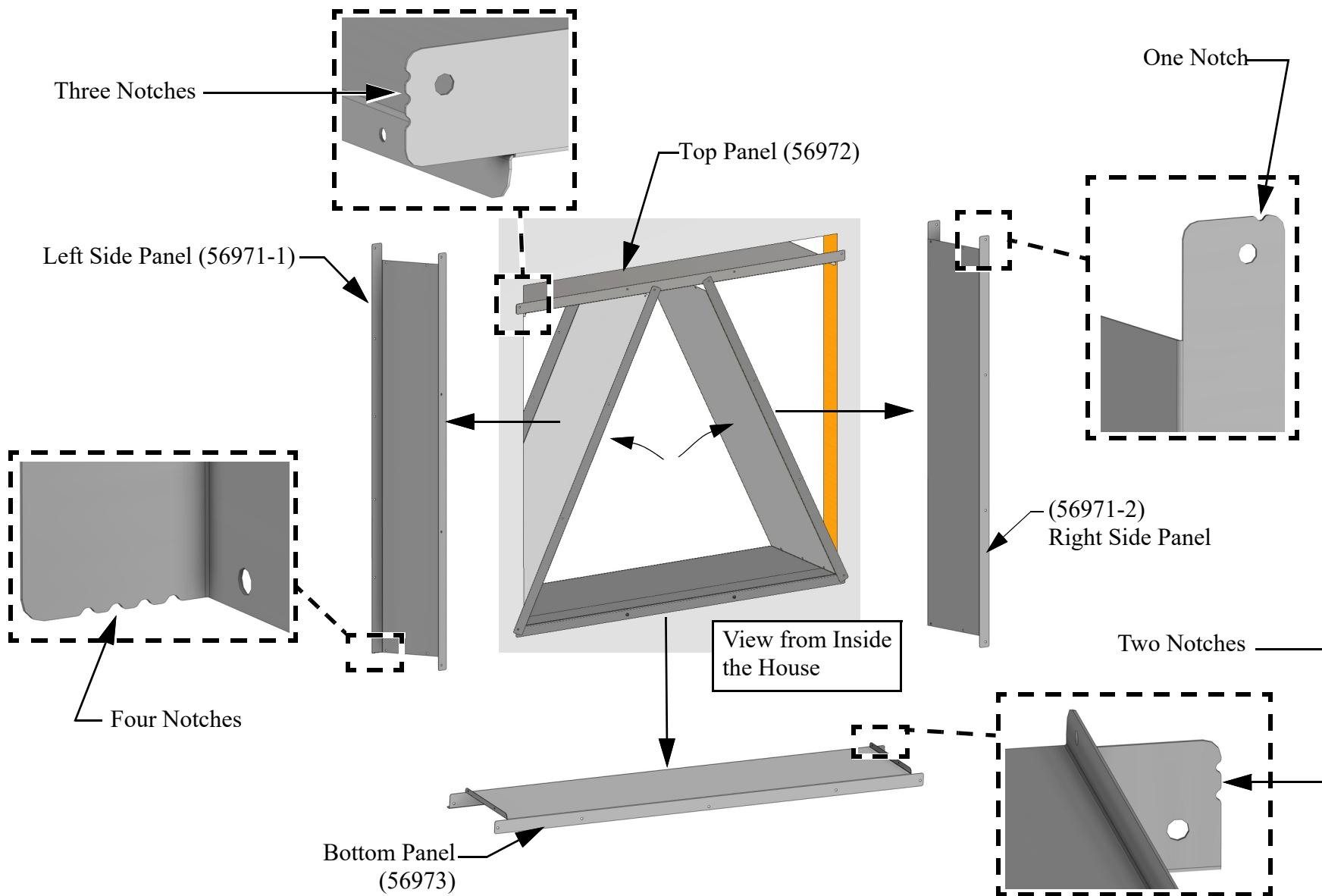
**Step 2:** Use four Self Tapping Screws (54683) to Fasten the Panels together using the holes provided toward the outside of the house **as shown**. Other four Screws will be installed after squaring.
