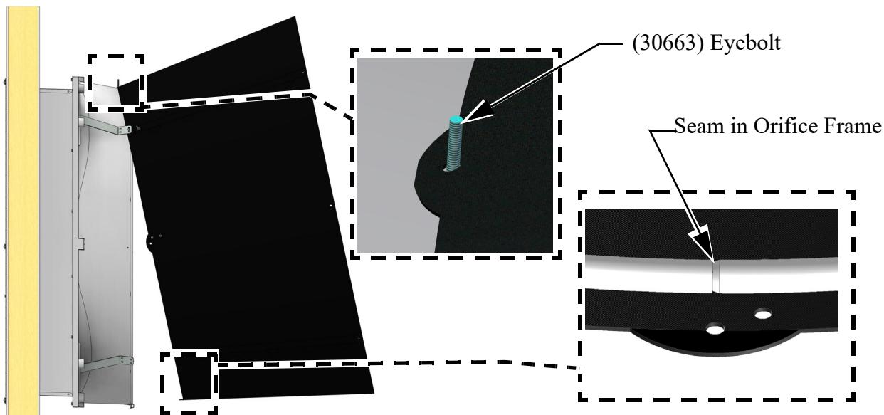
**Step 2:** Attach the Cone to the Shroud with 5/16 Flg. Nuts (46764) as shown
