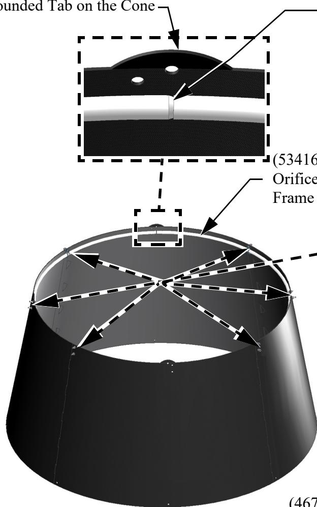
**Important!** Line up the Seam in the Orifice Frame with one of the rounded Tabs on the Cone.
