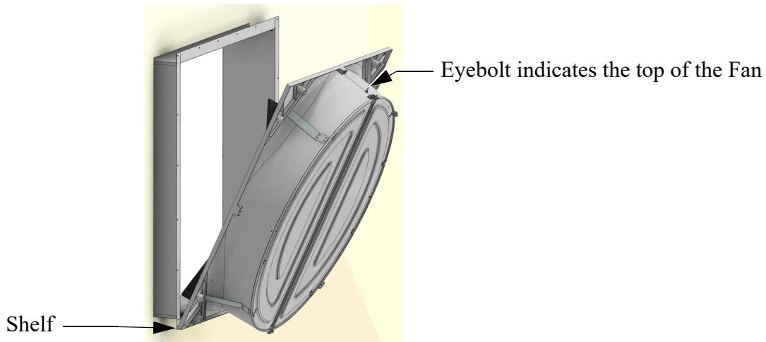
**Step 2:** Attach the Shroud to the Extension Box Panels with 20x 1/4-20 x 7/8" SS Bolts (4404-17) and 1/4-20 Flange Nuts (46298) **as shown**.
