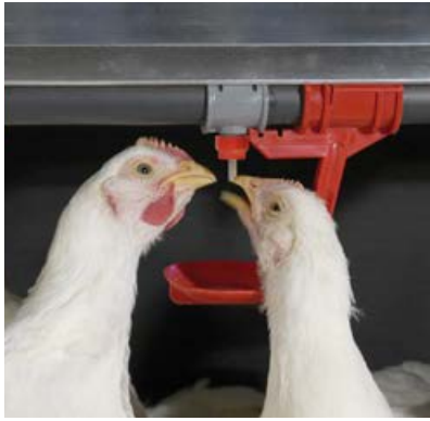
Catch Cup option for High Flow and Super High Flow systems.
